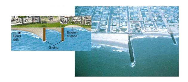
Sand deposition is greatly increased on the upcurrent side of the groin
